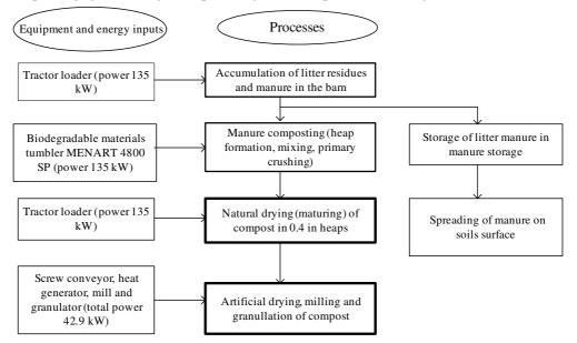
Fig. 1. Technologies for composting, granulation and surface spreading of cattle manure
