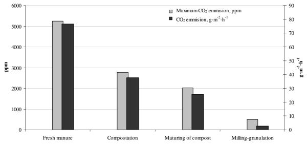
Fig.2. Measured carbon dioxide (CO<sub>2</sub>) emissions from technological operations of milled compost and granule production
